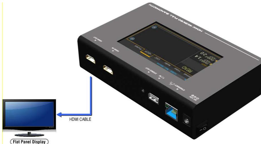
When MS-5005 set as transmitter, it can transmit HDCP encrypted video. MS-5005 also provides three modes (HDCP 1.4 / HDCP 2.2 / no HDCP) for you to select. If user wants to transmit HDCP encrypted video again, please select the Auto-Restart button.
